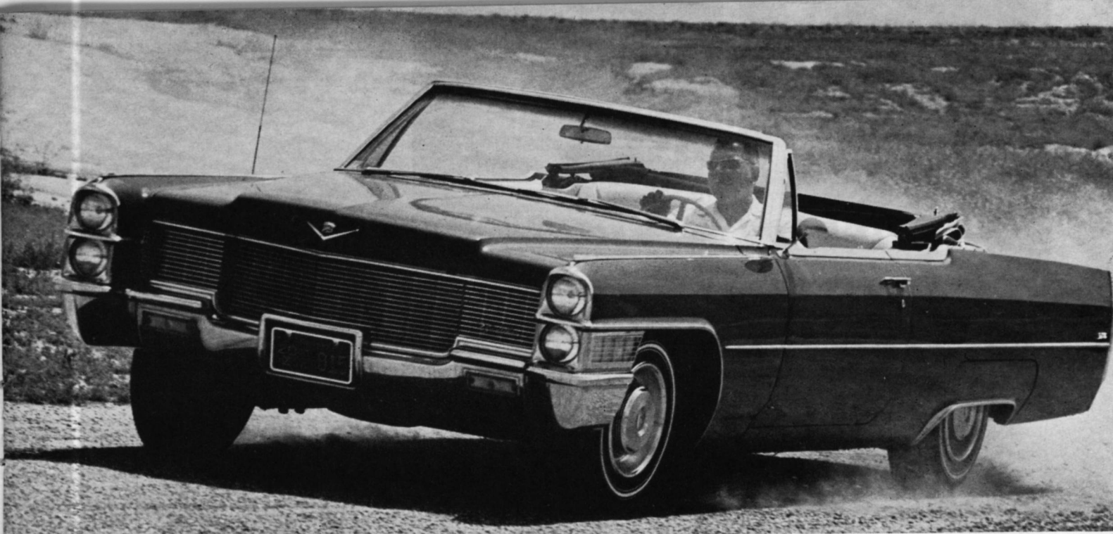
WIDENED TREAD AND LOW-PROFILE 9.00 X 15 TIRES IMPROVE CORNERING STABILITY, ALREADY RELATIVELY GOOD FOR A 4800-POUND CAR.
