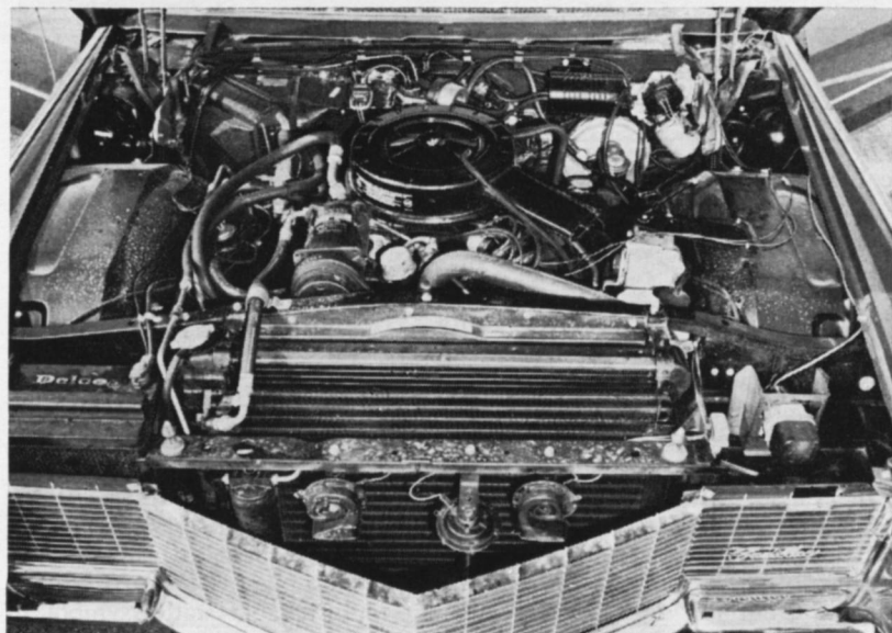
Numerous power-consuming accessories call for very busy engine compartment. Extra capacity of cross-flow radiator and condenser stops overheating.
